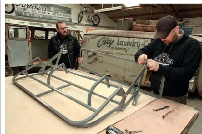
**08** The two hinges and both lower and rear seat frames should now be united and nipped up tight. Flip the seat over so it's resting on its rear frame and extend the hinge so that sections 3 and C are exposed at the bottom
