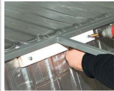
**19** To add some extra support to the back of the bed, Nick then made a stop out of some 50mm carcassing / sawn timber. Go very carefully here with the drill as on almost all Splits and all Bays the fuel tank sits right behind here. Ensure the place screws to hold this in place are suitably short
