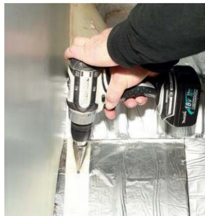
**15** With the positions accurately marked, bust out your best stepped hole cutting drill bit. Don't make the holes larger than the diameter of your bolts and ensure your tyres are clear of the 'arches before you puncture them. Don't forget to rust proof the bare metal edges of the holes with a suitable primer or rust preventative treatment
