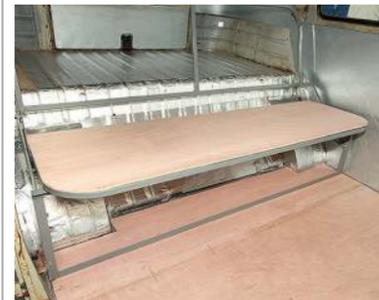
**20** The bed comes with two 9mm ply boards that form the base and back rest of your seat. Nick radiused the corners as shown freehand using a jigsaw. If you have never done this job before, we suggest you make a stiff card template, then flip it over so both corners match
