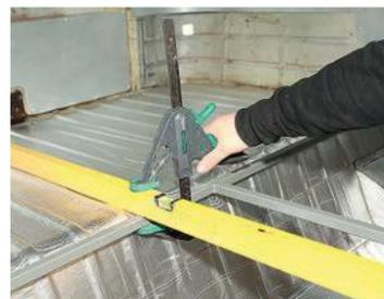
**13** Nick then unfolded the bed to ensure it sat straight and checked with a level. Rusty Lee's tag line, 'Sleep like a King' only applies if you put the bed in straight! Quick grips ensured it remained true
