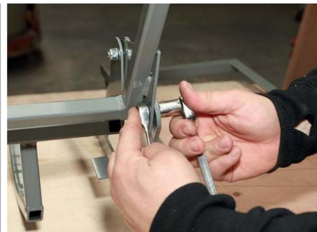
**07** Screw on the Nyloc and then tighten with the 13mm and 17mm socket / spanner. Repeat on both sides
