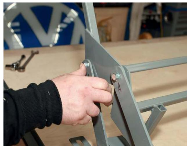
**06** Insert the next bolt through both section 2 and B on the left and right hinges into the back rest plate. Don't forget those washers between any metal surfaces
