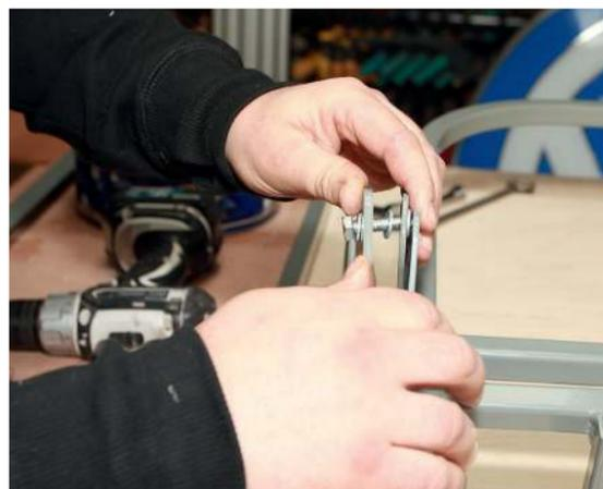
**03** As you're looking at the front of the seat, slot the first pair of the M8 bolts through the hinge with markings 1 and A. Don't forget to add the supplied washers both outside and inside the hinge as shown
