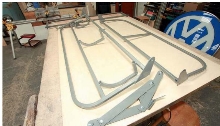
**02** Lay the bed sections out and acquaint yourself with the left hand and right hand-specific parts. Lee kindly writes on the bed frame and hinge sections in pen - 1, 2 and 3 on the left, A, B and C on the right. Altogether you should have five separate metal pieces to make up the bed
