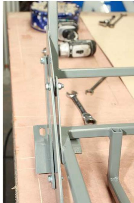
**10** After ensuring everything is nipped up nice and tight, stand the seat up to inspect your handiwork. You can see here how the washers are a vital part of the design as they permit enough room for the hinges to slide without interference.
