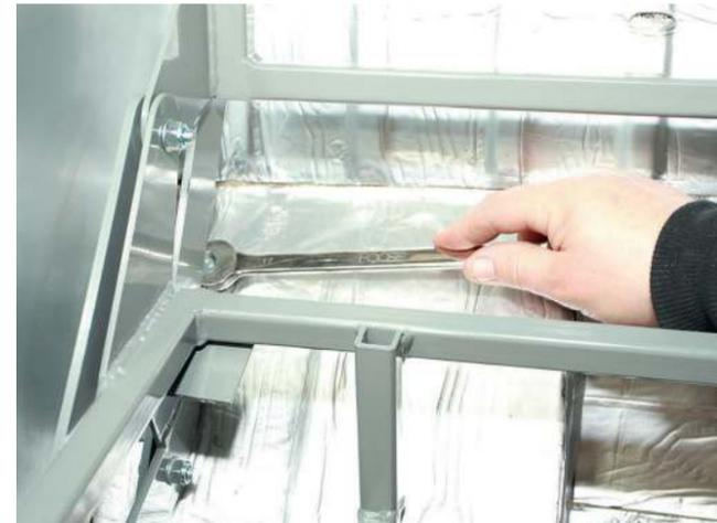
**17** With the help of your able assistant, wrestle the bed back into position and drop the bolts through the holes. What you can't see here is that Lee is underneath the Van with the socket ready to nip up the Nyloc from below. Repeat for the other side
