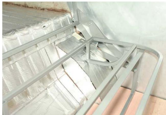
**12** Position the seat roughly upright so the bolt-in feet are level with the wheelarches. We used a strip of masking tape to avoid damaging the sound deadening, and also so we could mark the position of the holes to be drilled for the M10 high-tensile bolts. It should sit squarely so the 'arches support it, and obviously be central in the load space
