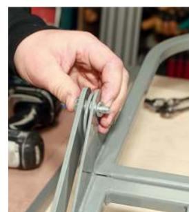
**04** Repeat this process on the other side and unite the hinge to the rest of the framework. Pass the bolt through the back rest fixing first, add another washer, then pass the bolt through the lower seat frame fixing and add another washer. You should end up with bolt head, washer, hinge, washer, back rest, washer, lower squab, washer, nut in that order
