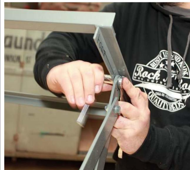
**09** Slide the third bolt through, again not forgetting those washers between each metal surface. Ensure the lower seat rest is pointing in the right direction. Tighten the nut and bolt using the 13mm and 17mm spanner / socket
