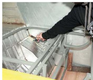
**14** Don't forget to check that the lower support structure is also straight using a set square. Mark the position of the holes to be drilled through the wheelarches for the M10 bolts to drop through
